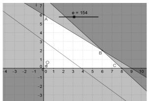
Move e on the slider then the line f will move parallel to the line 40x + 50y = 0. Observing the values, we can see e reaches its maximum value when the line f still cuts the quadrilateral OABC at 340. Now the line f go pass B(6; 2).
